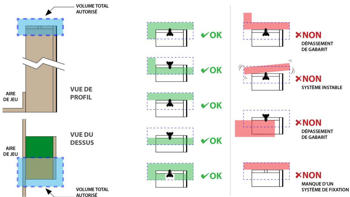
Figure 13 - How to install a central tracking device
