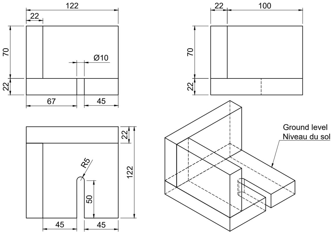
Figure 30 – Left fixed beacon support
